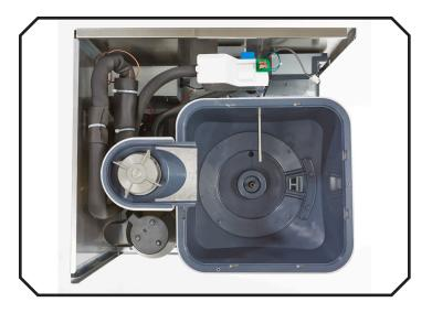
29. Wash the sink / drip tray and grill with the sanitizer solution. Pour remaining sanitizer into the bin and sink. Do not overfill bin.
