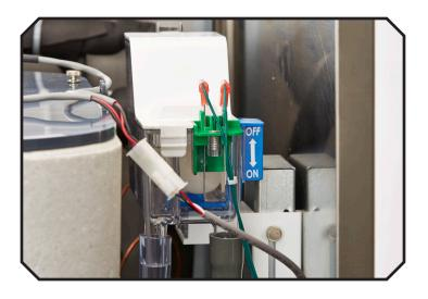
32. Return the chute cover, dispense rotor and agitator to the inside of the storage bin. Secure with the original fasteners.
