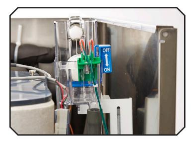
11. Remove dispense bin cover, but keep photo eyes connected to harness.
