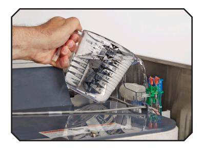
18. Drain the water from the water system by pulling the reservoir drain hose from its plug and return it to the plug when drained.
