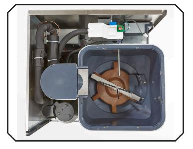
33. Return the ice dispense chute and water reservoir cover to their original positions and secure them with their original fasteners.
