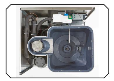
28. Wash the ice discharge chute cover, ice sweep, metal area below the ice sweep and ice dispense chute with the sanitizer solution.
