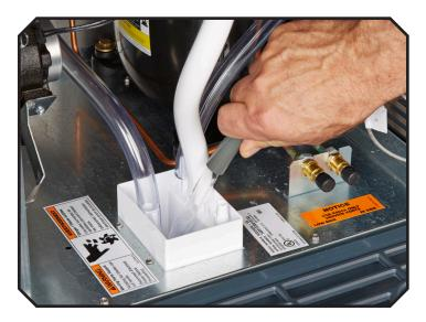
31. Loosen thumb screw holding water reservoir to post and lower the water reservoir to the top of the slot, retighten thumb screw.
