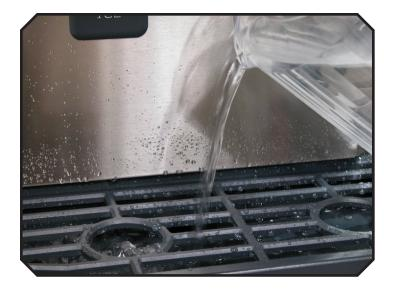
30. Drain sanitizer from ice making system by pulling reservoir drain hose from plug and return hose to plug when drained. Repeat with clean water.
