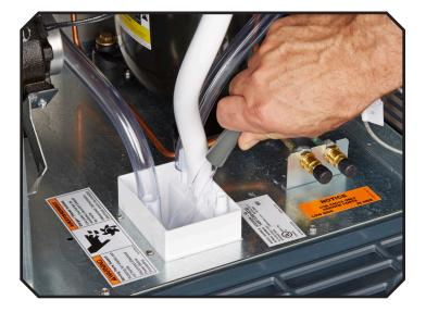
19. Mix a solution of 4 ounces of ice machine scale remover and 16 ounces of potable water. Use this scale remover solution to washout the water reservoir cover, ice discharge chute, ice chute cover, ice delivery chute, storage bin cover and inside of the ice storage bin. Also wash the sink /drip tray and grill with this solution. Pour half down the bin drain and the rest into the sink / drip tray to flush out their drains.
