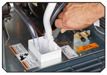
5. Remove reservoir cover and fill with hot (110-120 degree F.) water, wait 2 minutes and drain water from ice making system by pulling reservoir drain hose from plug and return hose to plug when drained.
