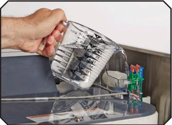
14. Push the Clean button. The unit will operate the auger motor for 30 minutes and then stop.
